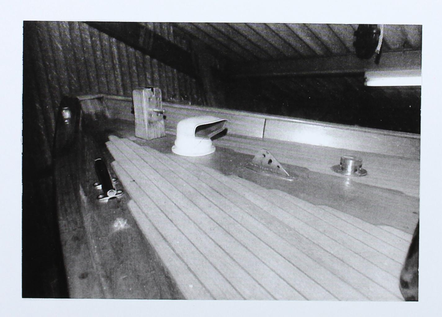
POSITIONING OF cleats, hawse pipe and ventilator.
